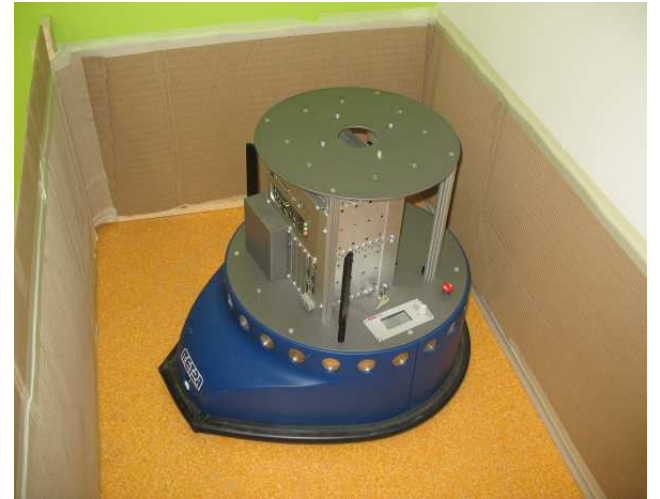
Fig. 2. Scitos G5 physical setup: the robot inside the box, walls are covered with corrugated cardboard for better sensor readings.
